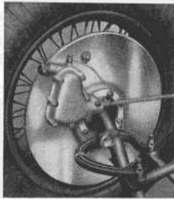
Self-Servo, cable-operated brakes.
