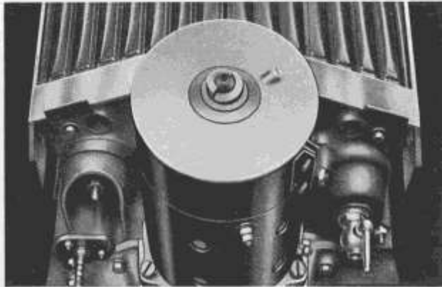
Radiator mounted on Engine.
